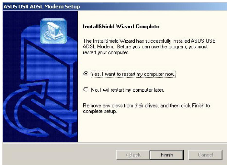
When the installation is complete, shut down your computer and connect your ADSL modem to your computer's USB port. Turn on the computer and wait until Windows XP starts or until you get to the Windows login screen. (**Note:** In Windows XP, you must login as an Administrator or have administrator rights for the installation to continue.)
